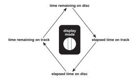
The information in the **time** portion of the display corresponds to the lighted LEDs to the right of the **display mode** button. After play begins, the display will reflect the last display mode you selected.
